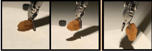
Fig. 9: Properties of raisins during debridement. Raisins are sticky and elastic, and a gripper that grips it by the edge often pulls it successfully out of the workspace (first two images). A type C error is when the gripper pulls it out using one tip (third image).
