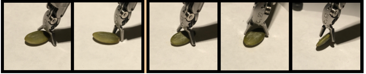
Fig. 8: Properties of pumpkin seeds during debridement. These seeds slide and rotate on the paper surface. Type A errors frequently result in the seed getting pushed out of the gripper’s control (first two images). This can also happen even if calibration is accurate and the dVRK ends up in a reasonable location. The third image shows a gripper initially in an excellent spot to grab the seed, but one tip can rotate the seed before it gets gripped (fourth image) which can cause it to snap out of control (fifth image). This is a type B error.
